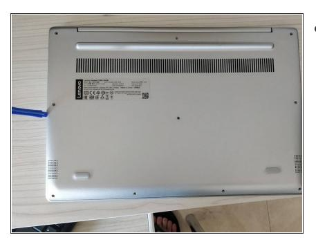
Use a plastic pry tool to open the device by sliding it gently around the laptop
