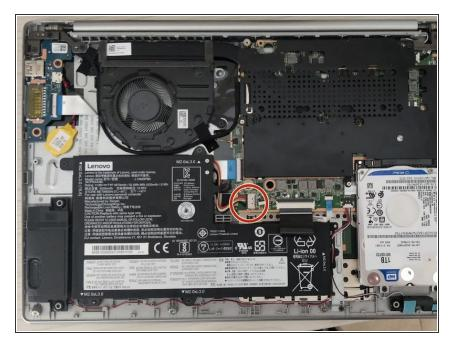
Using a spudger gently push the plastic connector to the left in order to disconnect the battery.
