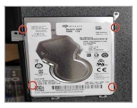
Remove the four screws as shown in pictures and remove the drive form the hard drive case. To reassemble your device, follow these instructions in reverse order.
