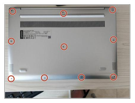
Remove 10 screws as shown in picture.
