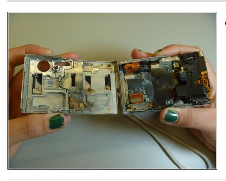
The front cover is now removed from the camera and the internal hardware is now exposed.
