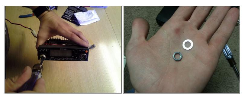
Below where the tuning knob was, there is a 7/16" nut that helps to secure the face plate to the radio. This needs to be removed to allow the face plate to be taken off.
