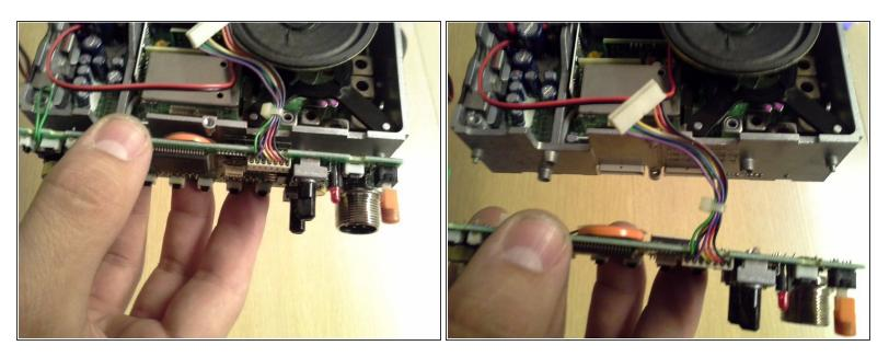
Pull the control board away from the radio body. It will be slightly more stubborn than the face plate was.
