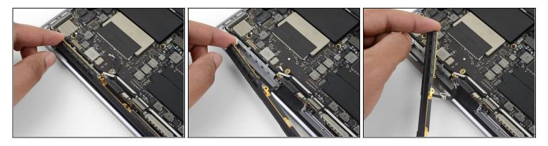
Carefully remove the antenna assembly, while simultaneously feeding the antenna cable bundle through the hole in the chassis.
