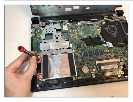
Remove the two 4 mm Phillips screws holding the hard drive adapter in place.
