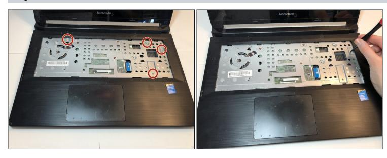
• Remove all four 3.5 mm Phillips screws underneath the keyboard.
