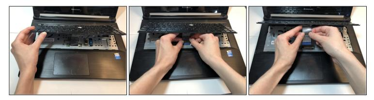
• Take out the keyboard by disconnecting the cable.
