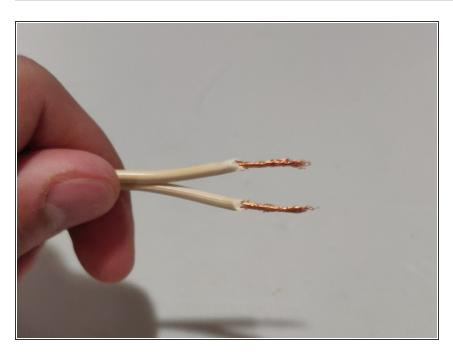
Use wire strippers to carefully peel the wire cord to expose 2 cm of wire.
