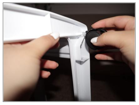
• Insert the glue coated metal tab of the wheel inside the hole.
