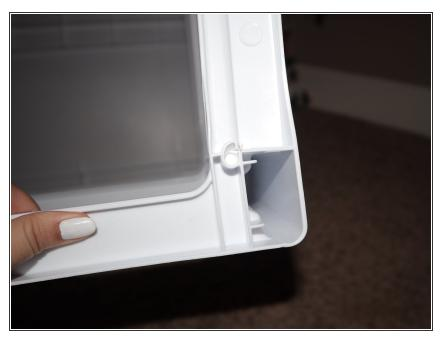
• Wait for the welded hole to cool down.
