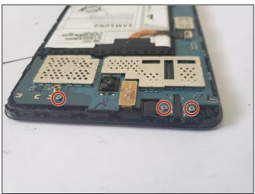
• Use a *Phillips #00* screwdriver to remove five *1.7 mm* screws from the top and bottom edges of the motherboard.
