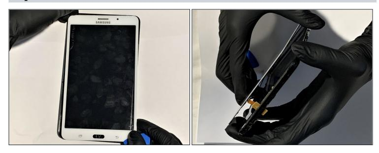
• Carefully lift up the digitizer. As you do, you will need to slide one of the press fit connectors through the midframe.
