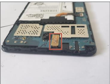
• Using the *flat end of a spudger*, unclip the press fit connections below the battery and at the top near the camera.
