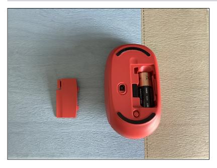
• Gently press the tab, and pull the door up and away from the body of the mouse
