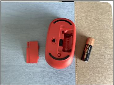
• Using your fingernail, pull up on the top of the battery and take it out of the slot.
