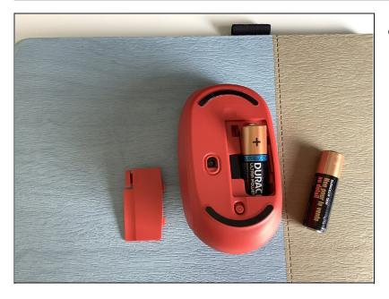
Slide the battery into the slot, and push down on it firmly. It will click into place.
