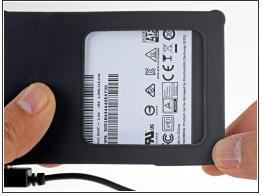
Stretch the remaining enclosure corners over the drive so that the silicone cover encapsulates the drive.
