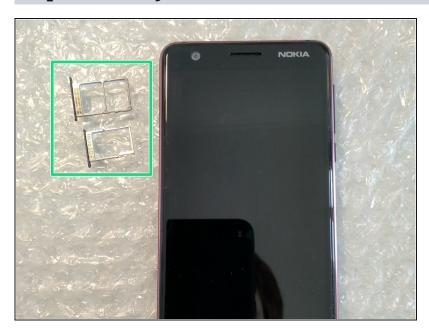
First, remove the SIM and SD card trays.
