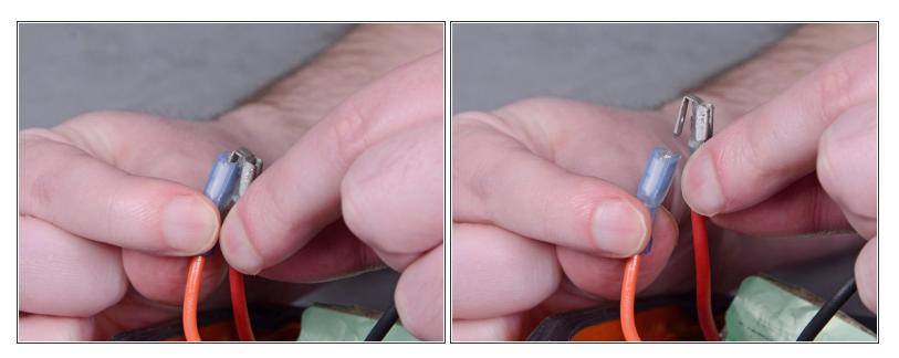
Be **very** careful with this connection, as even minimal bending can break the metal conductor in <u>half</u>.
