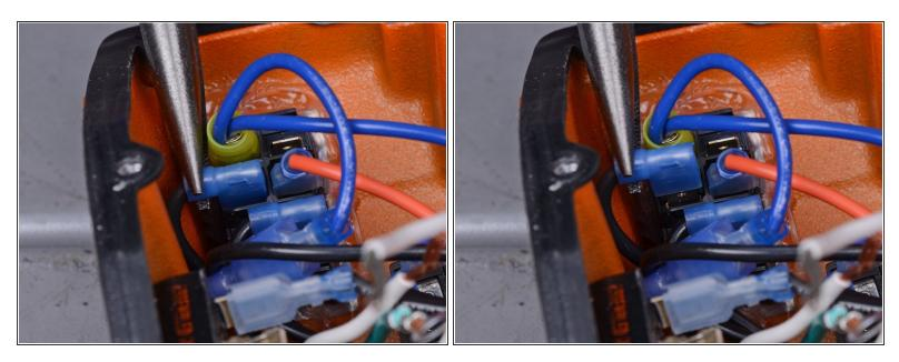
• Remove the black wire from the switch assembly.
