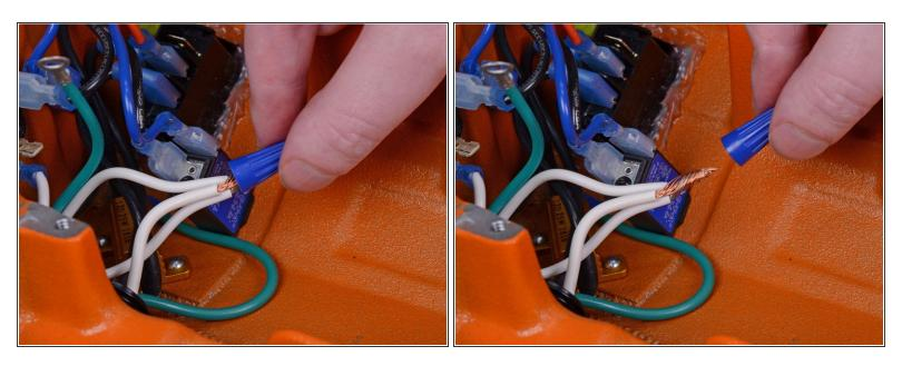
• Remove the twist-on wire connector.
