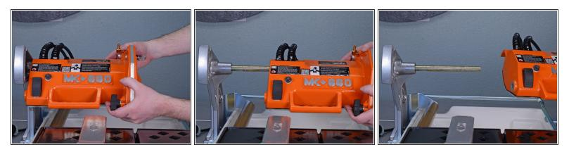
• Pull the entire cutting head straight off the shaft holding it in place.
