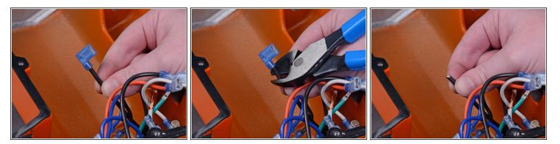
• Use wire cutters to cut the angled plug off the end of the black wire so it can slide out of the power cord opening.
