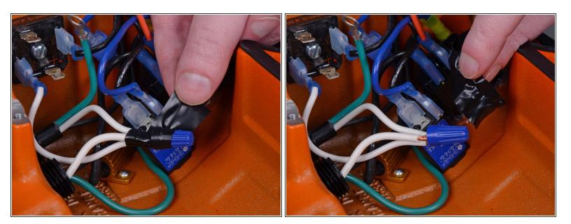
• Remove the electrical tape from the twist-on wire connector connecting the three white wires.
