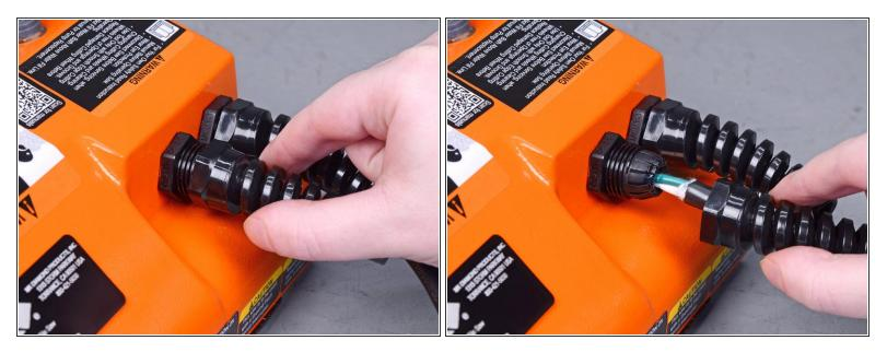
• Pull back the flex guard from the cutting head chassis.
