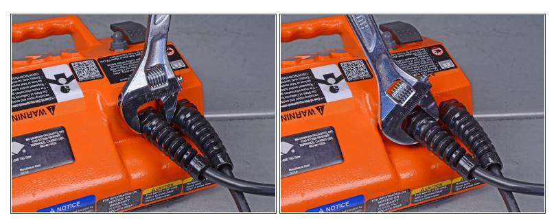
• Use an adjustable wrench to loosen the hex nut closest to the wall plug side of the power cord.
