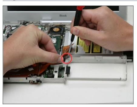
Peel back the orange ribbon cable to reveal a single Phillips screw. Remove this screw to free the optical drive from the metal framework.
