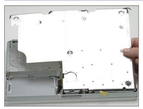
• Lift the bottom shield off.
