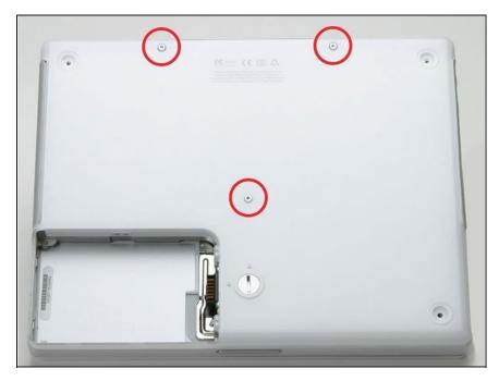
Remove the one 10 mm and two 20 mm hex screws using a 2mm hex. Alternatively, a T8 Torx screwdriver key will do.
