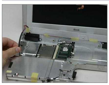
Lift the upper case off completely and disconnect the red and black speaker cable from the logic board. As before, make sure you're pulling only on the connector and not on the socket.
