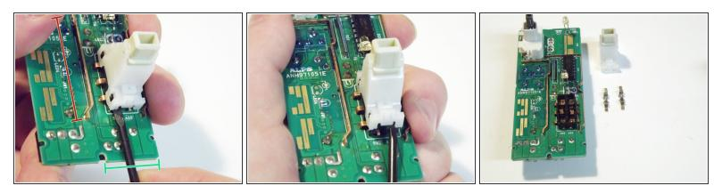
• Using a thin spudger, carefully pry these two latches off of the lever.
