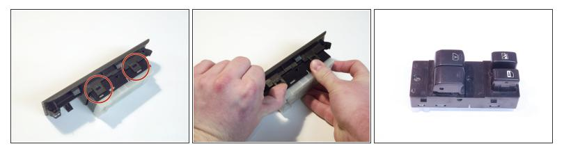
• Pry the marked latches off on both sides to remove the molding around the button assembly.
