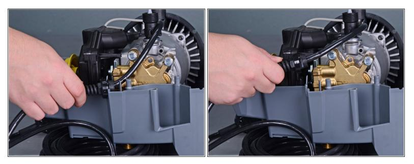
• Slide the power cord strain relief out its notch on the plastic housing.
