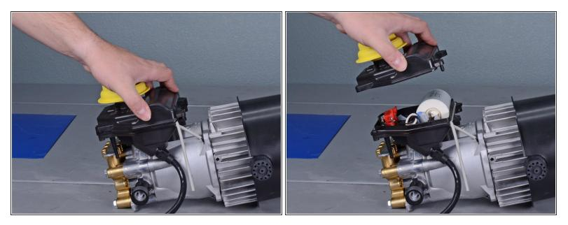
• Lift the cover off of the electrical box.
