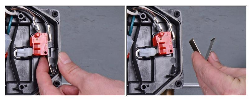
• Remove the plate spring from the electrical box.
