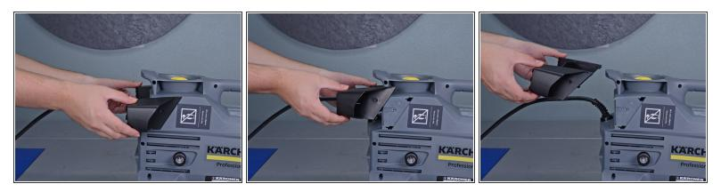
• Unclip and remove the plastic feet.
