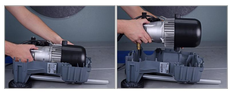
• Lift the motor assembly out of the plastic housing and set it aside.
