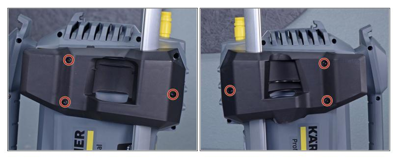
Use a T15 driver to remove the six screws securing the top black plastic panels on either side of the device.
