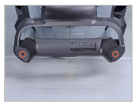
Use a T20 driver to remove the two 55mm-long screws securing the hand grip.
