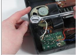
Remove the fasteners using an 11 mm socket wrench.
