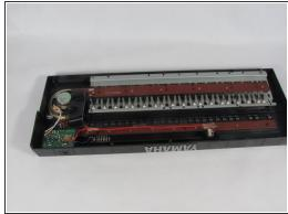
Rotate the keyboard to get a better angle with the soldering iron.
