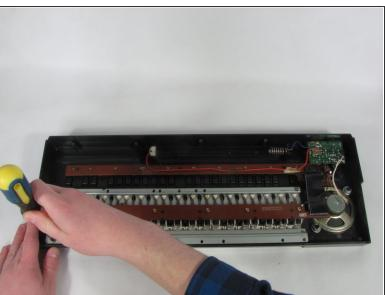
Replace two 9.0 mm Phillips screws to keep the keys from falling out while working on this device.
