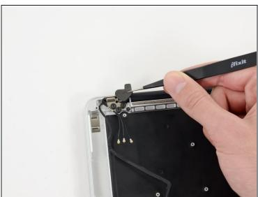
• Use a pair of <u>tweezers</u> to lift the rubber hinge covers up off the right and left display hinges.
