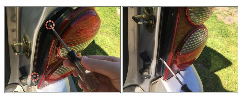
Use the T-20 Torx screwdriver to unscrew the two screws holding the tail light cover.
