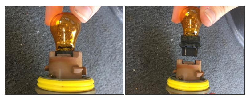
Grasp the lightbulb and pull it out of the socket.
