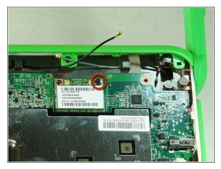
• Remove the black 4mm Phillips #1 screw holding the wireless card in.
