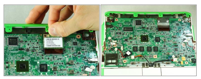
• Remove the wireless card from the laptop by gently sliding it out of its socket.
