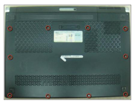
Remove the lower panel of the laptop by loosening 10 screws. Note that the screws do no come out of the back panel.
