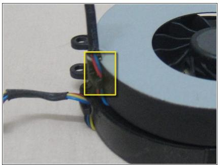
Unpack the new fan. Make sure the power wires are fixed in the hook provided.
