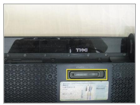
Remove the battery by sliding the battery lock switch
