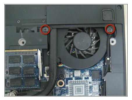
Remove two screws which holds a smaller back panel covering only the heatsink
