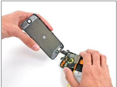
Remove the display assembly from the iPod.
