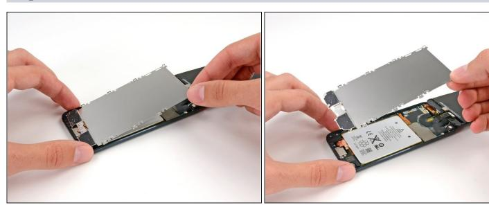
• Lift up and remove the LCD plate from the iPod.
