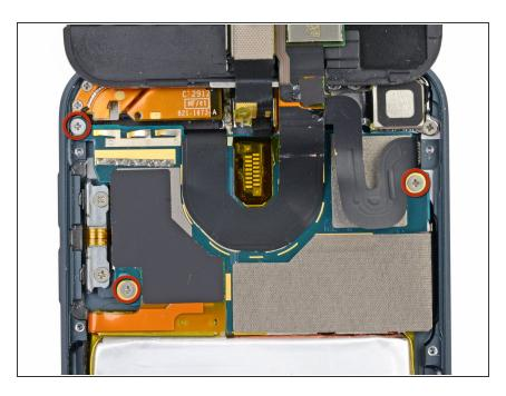
Remove three 1.6 mm #000 Phillips screws securing the logic board to the rear case.
