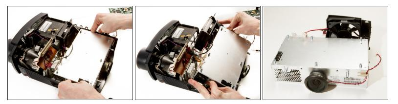
Use your thumbs to pry the sides of the external shell away from the power supply so it can be lifted out.
