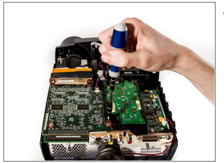
Remove the four T10 Torx 8.5 mm screws holding the DLP board in place.
