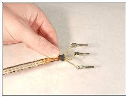
Lift the wires and prongs out of the clamshell.
