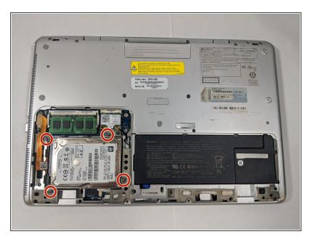
Remove the four 3mm screws using the Phillips #1 screwdriver.
