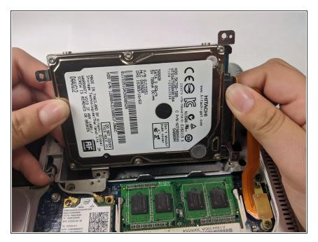
• Lift out the hard drive and unplug the orange ribbon wire.
