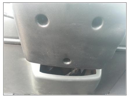
Remove the three "torx head" screws to release the plastic cover from the steering column.
