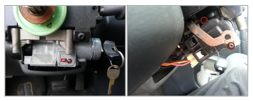
• Sit in the car facing the steering wheel. Lean to the left to locate the two "torx head" screws on the ignition. Remove these.
