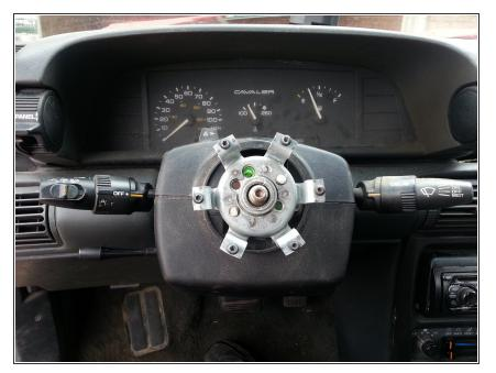
Locate the six "torx head" screws that hold the steering wheel to the steering wheel hub. Removing the screws is not necessary but will make the job easier.
