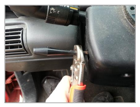
Using locking pliers, unscrew the tiltadjusting lever. Wrap a shop towel or dish cloth around the lever to prevent scratches.
