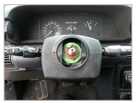
Remove the steering shaft nut and pull off the steering hub. A steering wheel puller may be required. Use caution as the steering hub may pop loose. Next, remove the two "torx head" screws behind the steering hub that hold the two plastic covers together.
