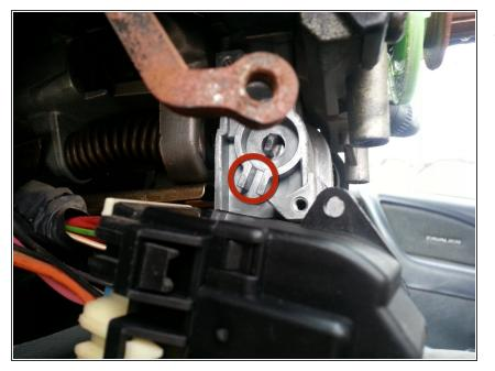
Tab A goes into slot B, marked in the photo. Also note that just above the red circle is the end of the ignition lock cylinder in the off position. If yours is not in the off position, it should be.
