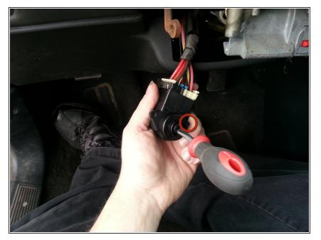
Using a flat head screwdriver, test the new switch. Do so by reconnecting the battery and turning the switch in either direction. The switch should turn smoothly and only kick back to the on position.
