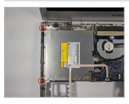
Remove the two 3mm screws using the Phillips #1 screwdriver.
