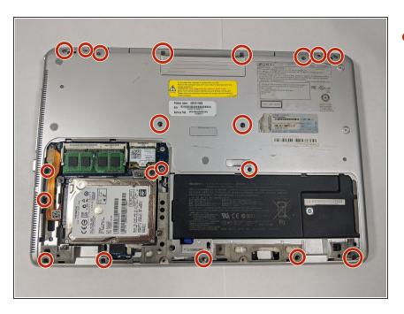
To loosen the keyboard, remove the twenty 5mm screws using the Phillips #1 screwdriver.
