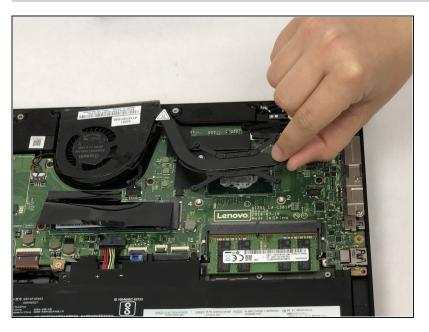
Using your index finger and thumb, gently pry the cooler from its mountings and remove the assembly.
