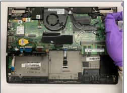
• Pull up on the 2 black tabs to remove the cords located along the hinge edge of the device.
