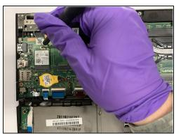
Using a Phillips #1 screwdriver, remove the 1.3 mm screw and set it aside.
