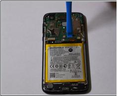
Using an iFixit opener tool, detach the fingerprint sensor and the other 5 cables from the motherboard.
