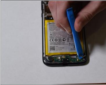
Using an iFixit opening tool, detach the cables from the charging port assembly.
