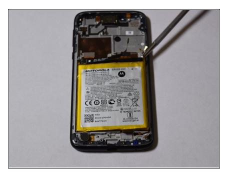
Pry the battery up now that the adhesive has been separated from the battery.
