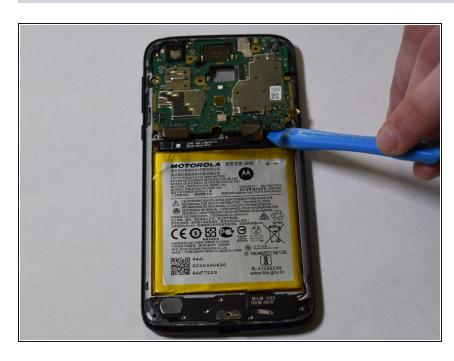
Carefully pry up the motherboard from the bottom with an iFixit opener tool.
