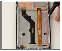
• Using a spudger, break both adhesive strips on the back side of the battery.
