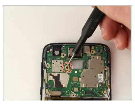
Remove the 0.4mm Phillips #00 screw from the motherboard with a 00 Phillips bit.
