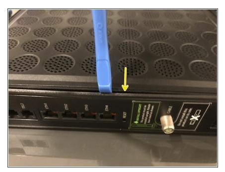
Take a pry tool and pull the cover off, on the side facing up from the last step. This is the side without the label.
