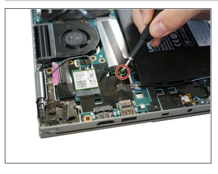
• Use a Phillips #0 screwdriver to remove one 6 mm screw.
