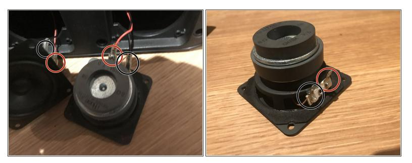
Remove the wires, which have different sockets, so they can't be mixed up.
