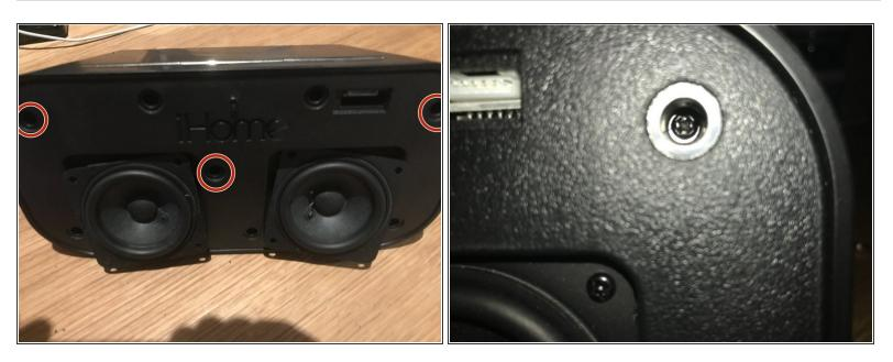
Remove these 3 screws, which were below the rubber inserts you removed earlier.
