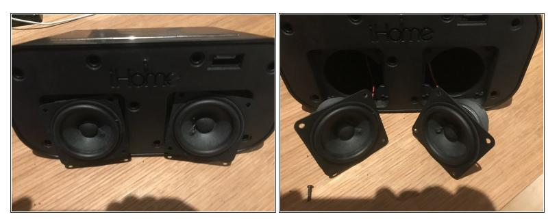
• The speaker can now be pulled out or removed by tilting the device.
