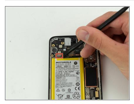
Remove the fingerprint scanner connector from the motherboard by levering the spudger underneath the connector corner.
