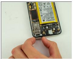
Use the SIM card removal bit to remove the SIM card tray.
