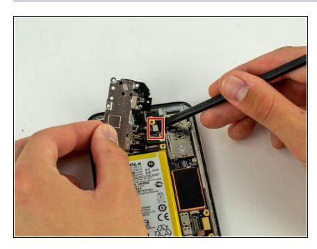
• Use a spudger beneath the right side of the connector to detach it.
