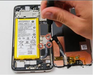
Remove three 2.7mm T3 Torx screws from the metal piece to the right of the battery.
