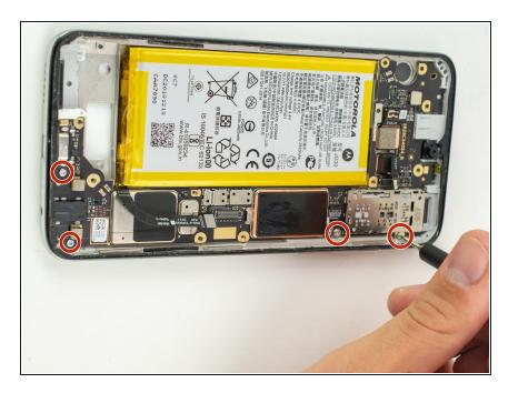
Use a T3 Torx screwdriver to remove the four 2.3mm screws from the bottom and right sides of the phone.
