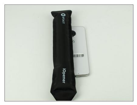
Use the iOpener or a heat gun around the edges of the phone to weaken the adhesive.
