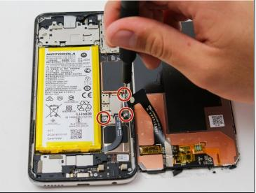
Remove three 2.7mm T3 Torx screws from the metal piece to the right of the battery.
