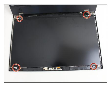
Remove all the screws holding down the screen.
