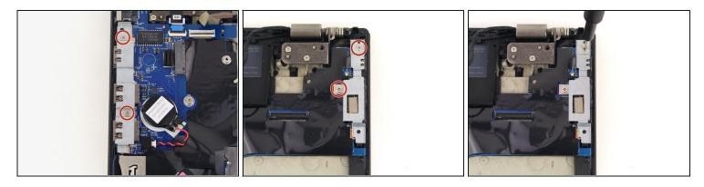
• Using a Phillips #00 screwdriver, remove the four 3.6 mm screws holding down the port brackets on the right and left sides of the motherboard.
