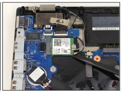
Using a spudger, pop off the gray and black coaxial cables from the Wi-Fi card.
