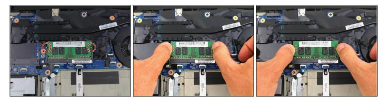
Pull the two tabs on either side of the RAM card outwards with your fingers.
