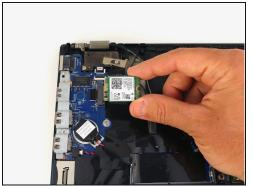
• Slide the Wi-Fi card out from the socket on the motherboard.
