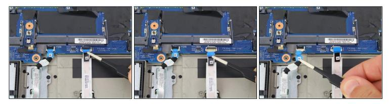
• Pull out the two ribbon cables with a pair of blunt nose tweezers.
