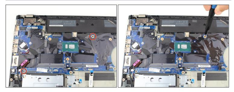
• Remove the two 3.3 mm screws from the motherboard with a Phillips #00 screwdriver.
