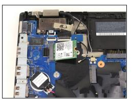
Using a Phillips #00 screwdriver, remove the 3.6 mm screw from the Wi-Fi card.
