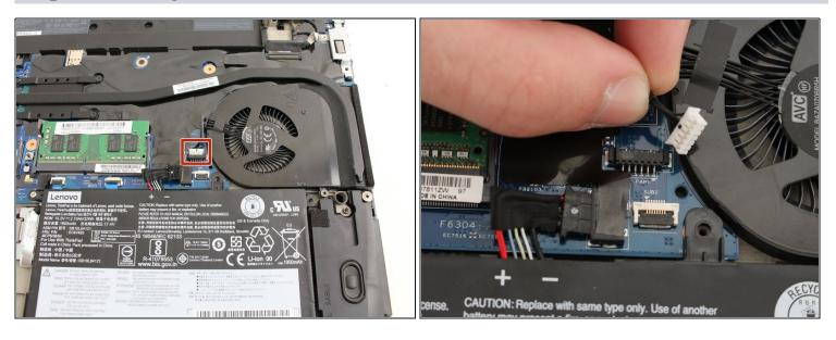
Unplug the cooling fan's cable from the the motherboard.
