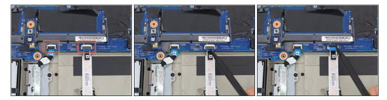
• Flip up the two ZIF cables for the trackpad and fingerprint sensor with the pointed end of a plastic spudger.
