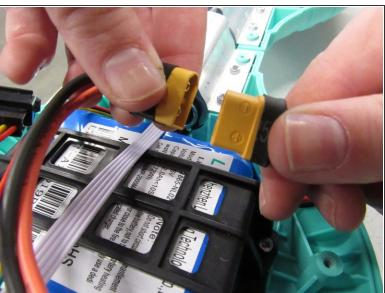
Disconnect the battery to prevent any electrical currents from coming through the wires.
