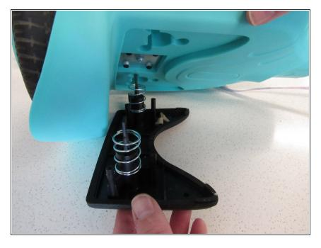
Remove the foot mats from the top of the board, which is facing down right now.
