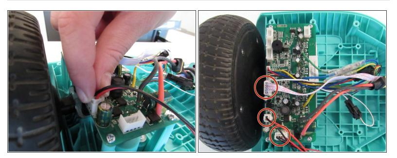
Squeeze and pull on the wires to detach them from the motherboard.
