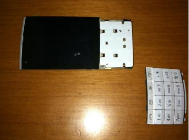
Remove the keyboard with a plastic opening tool.
