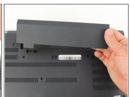
Pull the battery directly out of the socket
