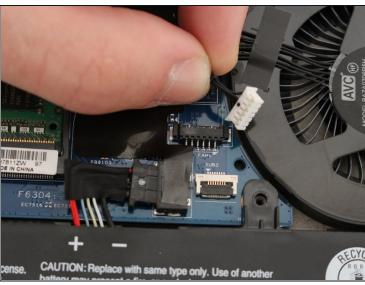
Unplug the cooling fan's cable from the the motherboard.
