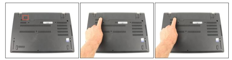
• Slide the switch on the left side of the battery to the left.
