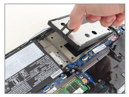
• Pull the hard drive case out of the slot using the tab.
