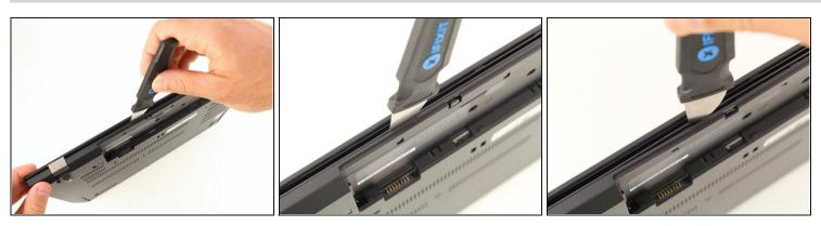
• Run a Jimmy along the crease of the computer all the way around, twisting it periodically to disengage the clips.
