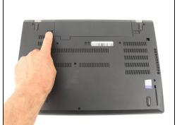
Slide the switch on the left side of the battery to the left.
