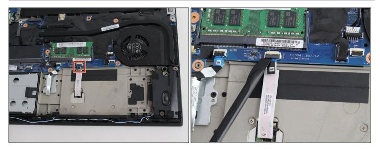
Using a halberd spudger, unplug the trackpad cable from the motherboard.
