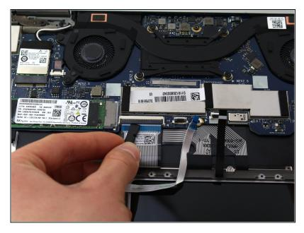
Use a spudger to remove the keyboard cable by flipping up the gray connector tab. Pull out the cable.
