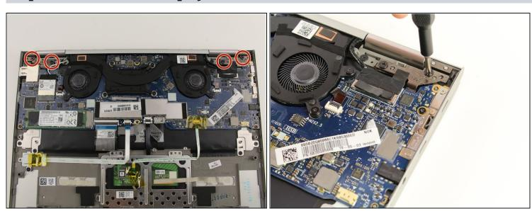
Use a Phillips #00 screwdriver to remove the four 4mm display hinge screws.
