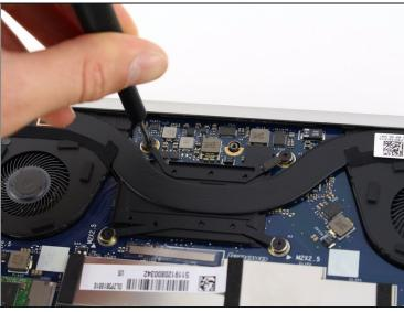
Use a Phillips #00 screwdriver to remove the eight 2.5mm screws securing the heat sink assembly.
