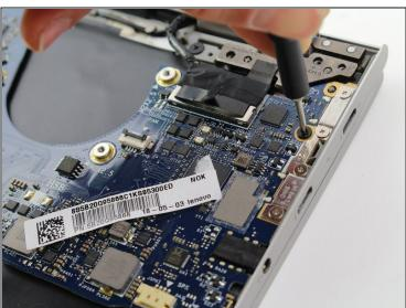
• Use a Phillips #00 screwdriver to remove the five 3.5mm screws securing the motherboard.
