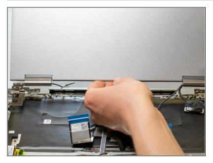
Lift the touchscreen back and up to unhook the hinges from the laptop frame.
