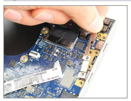
Lift the bracket up from the motherboard and place aside.
