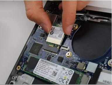
Gently slide the LAN card straight out of the motherboard connector.
