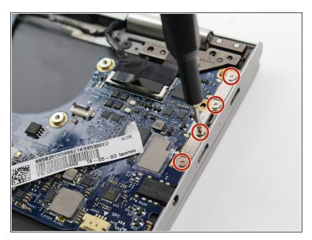
Use a Phillips #000 driver to remove the four 3mm screws holding down the connector bracket.
