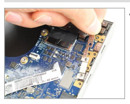
Lift the bracket up from the motherboard and place aside.
