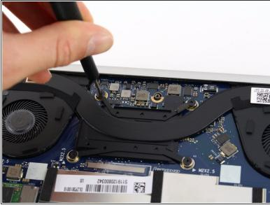
• Use a Phillips #00 screwdriver to remove the eight 2.5mm screws securing the heat sink assembly.
