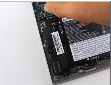
Remove the four 3.5mm Phillips #0 screws securing the battery.
