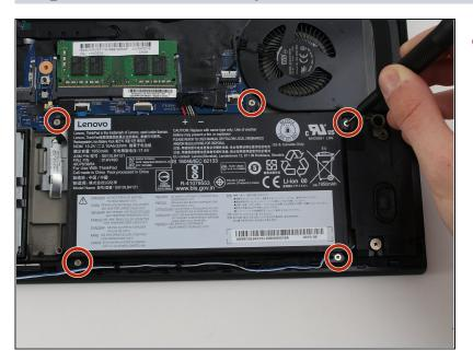
Using a Phillips #00 screwdriver, remove five 3.7 mm screws holding down the battery.
