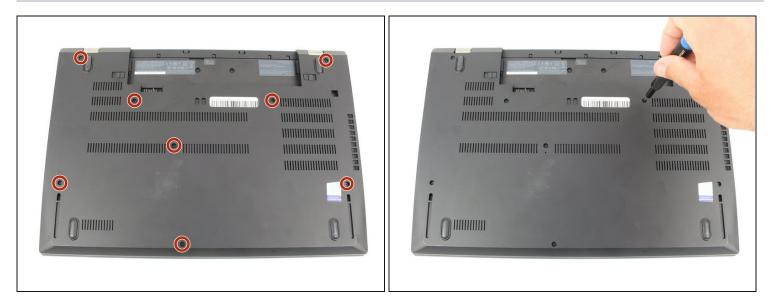
• Using a Phillips #00 screwdriver, unscrew the eight 3.3 mm captive screws on the bottom of the laptop.
