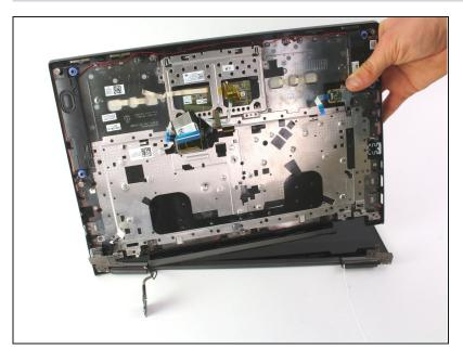
Pull the keyboard up away from the screen. After the display and antenna wires have been moved, the keyboard should easily come apart from the screen.
