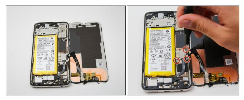
• Remove three 2.7mm T3 Torx screws from the metal piece to the right of the battery.
