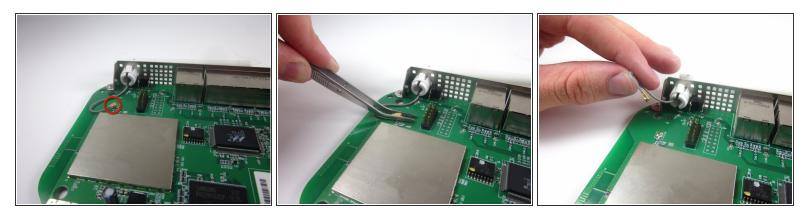
• Use tweezers to gently pull the metal bracket that connects the antenna to the motherboard.
