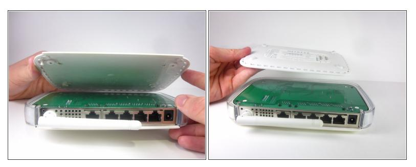
• Lift the lower case straight up from the rest of the router.
