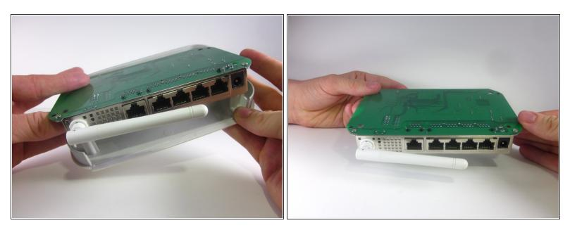
• Separate the motherboard from the top shell by lifting it straight up from the router.
