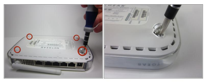
Unscrew the 4 11.8 mm T-8 Torx screws from each corner of the device.
