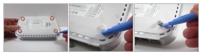
• Use the plastic opening tool to carefully lift the rubber stops in each corner.
