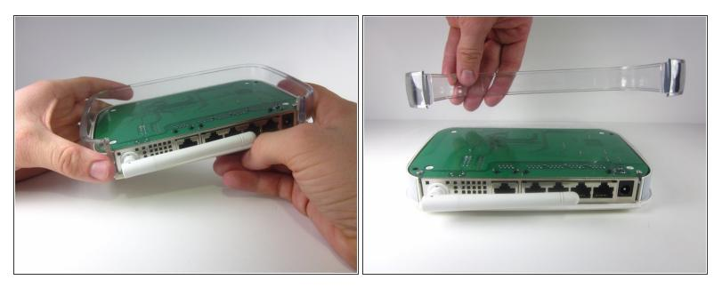
• Remove the clear plastic casing by lifting it straight up from the router.
